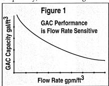
The removal rates with respect to EBCT are based on the "half length" concept. If a retention time of x minutes results in the removal of 50 percent, then a retention time of 2x minutes results in 75 percent and 3x equals 87.5 percent. Assuming 95 percent as breakthrough for a particular application, one must theoretically provide the equivalent of five half lengths. If half length is determined to be 60 seconds, an EBCT of five minutes will give 95-plus percent adsorption (see Table 1).
