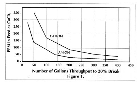
tridge represents only about 1/40th of a cubic foot of resin. At flow rates of 0.5 to 0.75 gpm (typical of counter-top filters), that is equivalent to 20 to 30 gpm/ft<sup>3</sup>! Resin manufacturers shy away from flows above 5 gpm/ft<sup>3</sup>. Do cartridges work at these high flow rates? The answer is yes. And, they work very well. The key is that they have to be properly de-
